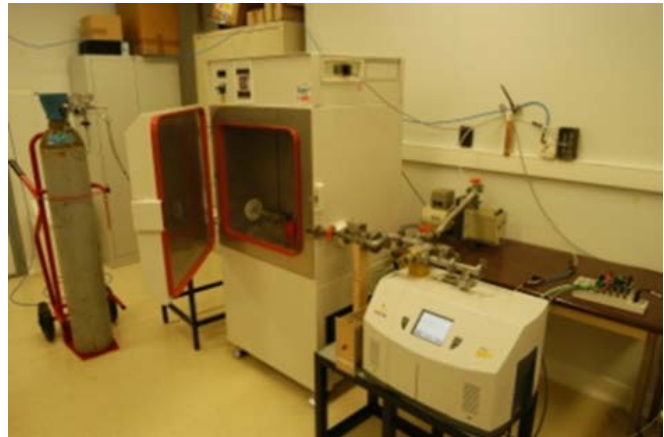
Banc de test raccords fluides
