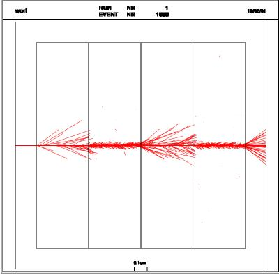
Cut in range: sampling: LAr(4mm) Pb(4mm). Protons 500 MeV.
