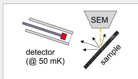
combination of cryogenic detector and scanning electron microscope
