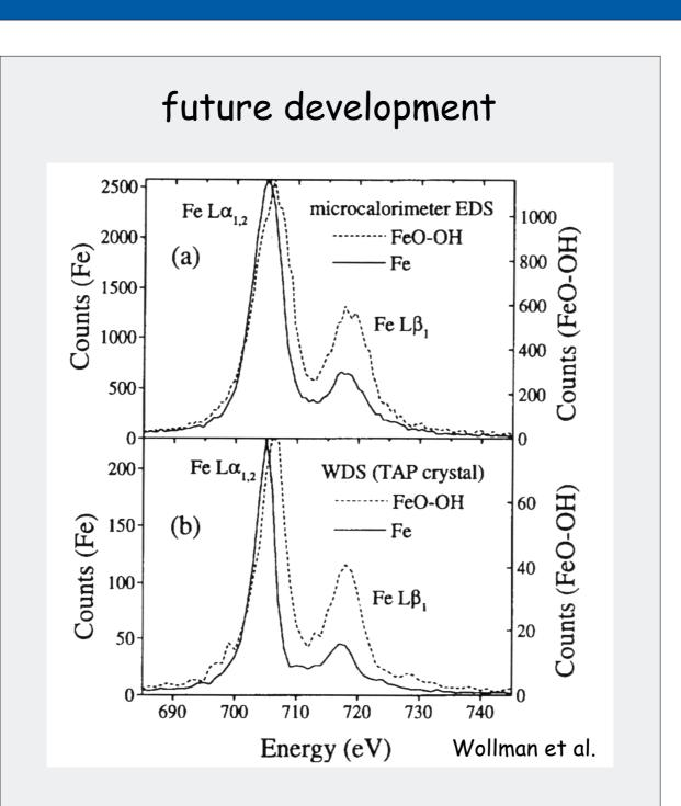
identification of chemical bonds by measurement of chemical shifts
