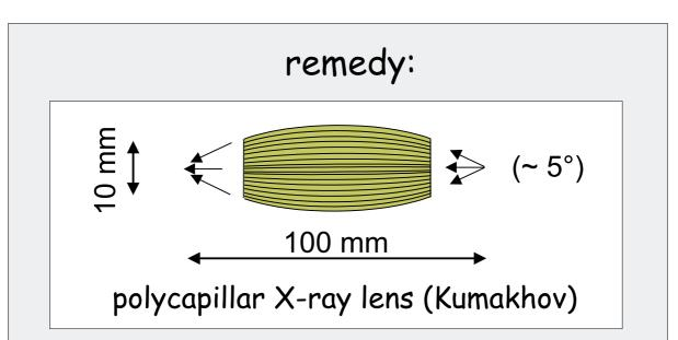
multiple total reflection inside polycapillars allows two-dimensional collimation of X-rays by very compact lenses
