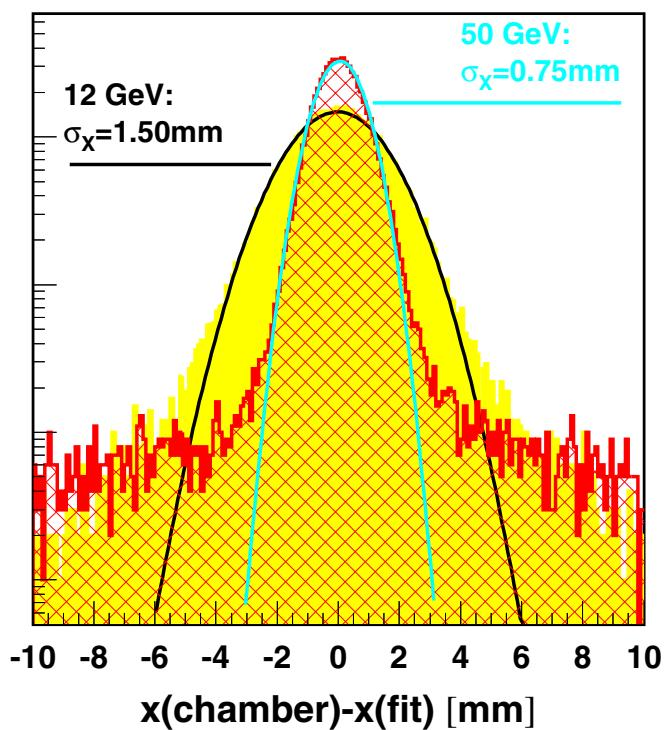
$$\text{position resolution: } \sigma_x = \frac{5\text{ mm}}{\sqrt{E[\text{GeV}]}}$$
