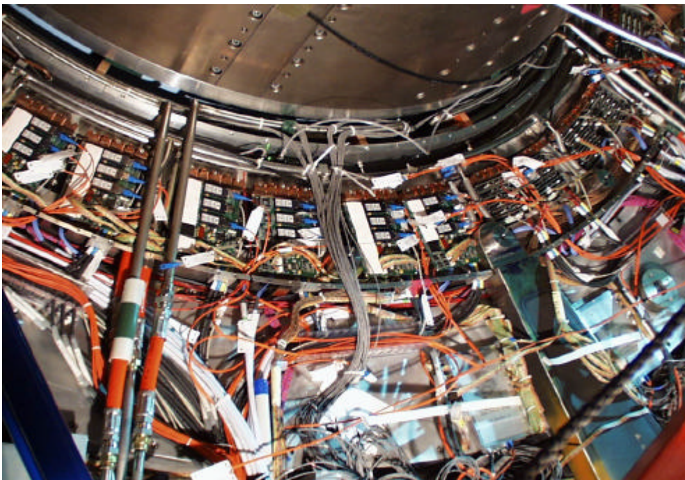
Front End Electronics 560 ADC boards 100 I/O boards
