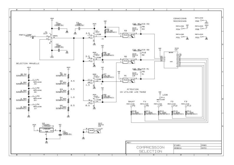
Whatever the type of external selection (manual or DAC), the selection voltage is compared to 4 threshold voltages (0,5V; 1,5V; 2,5V; 3,5V) performed using resistors bridge. So, at the output of the 4 comparators, we have a 4 bits digital word, which can be decoded to control the relays (cf. ABCD).
