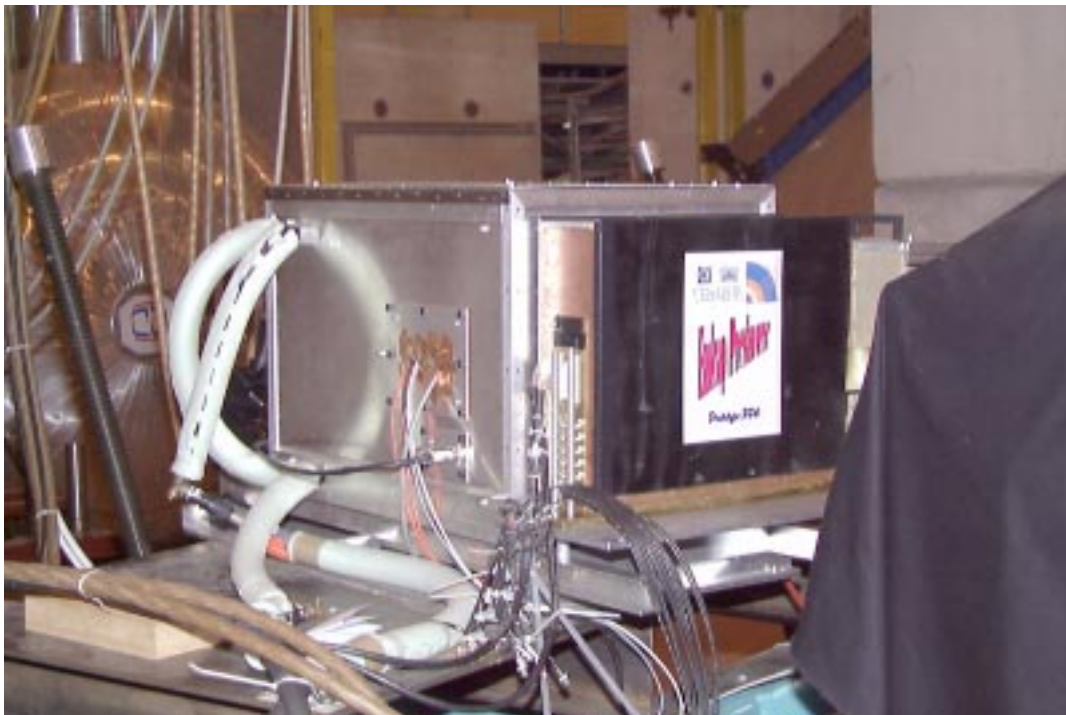
Figure 6: Photograph showing the preshower prototype placed in front of the ECAL endcap box. The complete system is situated on the moving table. The beam enters from the right.
