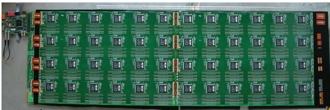
Figure 10. Photograph of two PCBs equipped with 24 HARDROCs each. The active area of a PCB is 32×48 cm 2 .
